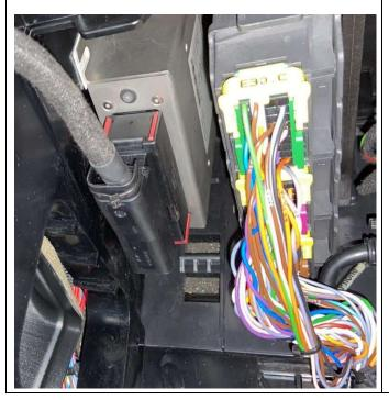
The RTA-ECU can be mounted at the passenger side of the central electric unit. Select a suitable free space and connect and fix in place.
