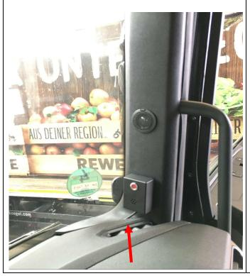
The signal box is mounted at the passenger side of the vehicle (A-column) at the same height as the rear view mirror so that the driver has it in his field of view while turning right.
