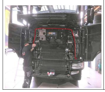
Cable positioning (highlighted in red), of the steering wheel sensor underneath the service hood of the Scania NGT in the vehicle cabin to the central electric unit. (see arrow in picture below).
