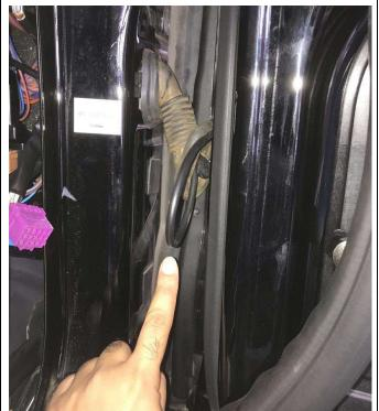
The radar sensor cable is positioned through the passage of the passenger door using a pull-cord or manually and then guided along into the vehicle interior
