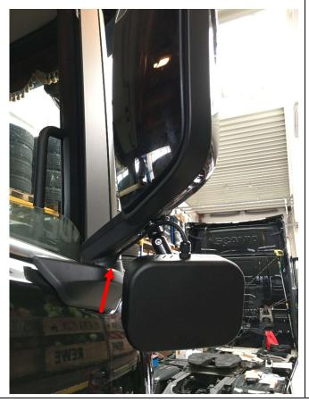
The radar sensor is mounted below the rear view mirror (mirror height above 2M) and the cables are positioned through the plastic mirror holder cover, (see arrow marker in the picture).
