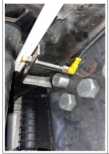
Photo with the measures of the mounting strip of the steering angle sensor.
