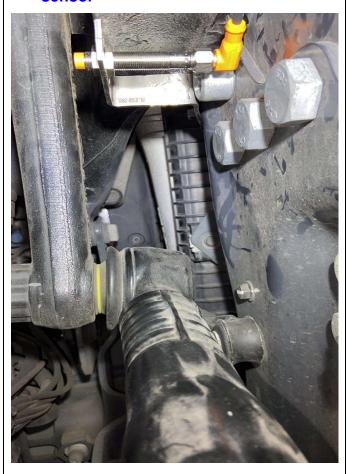
The steering wheel sensor is mounted in the vicinity of the steering rod. This is situated at the left front wheel (driver side).
